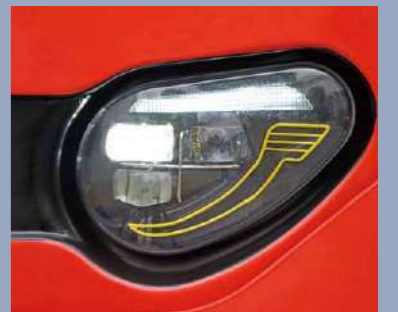
LED headlight has the head light and dipped light functions. The front turn light utilizes the latest stream light technology
