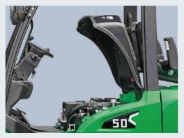
The hood (with a self-locking gas spring) can be opened at a large angle facilitating the maintenance and replacement of the battery.
